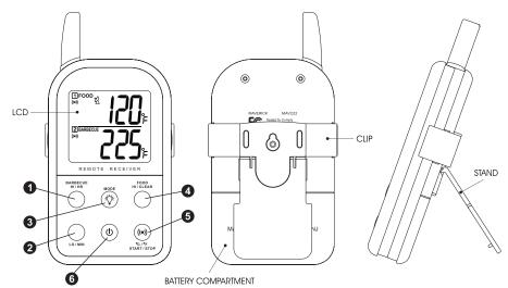
LCD (Liquid Crystal Display) - Displays all icons, temperature and time.
